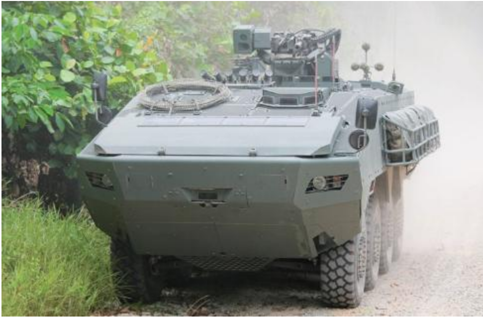
Terrex ICV of the Singapore Armed Forces fitted with an EOS R-600 RCWS armed with 40 mm AGL and 7.62 mm co-axial MG. The latter has an ABM capability. (SAF) 1347972
