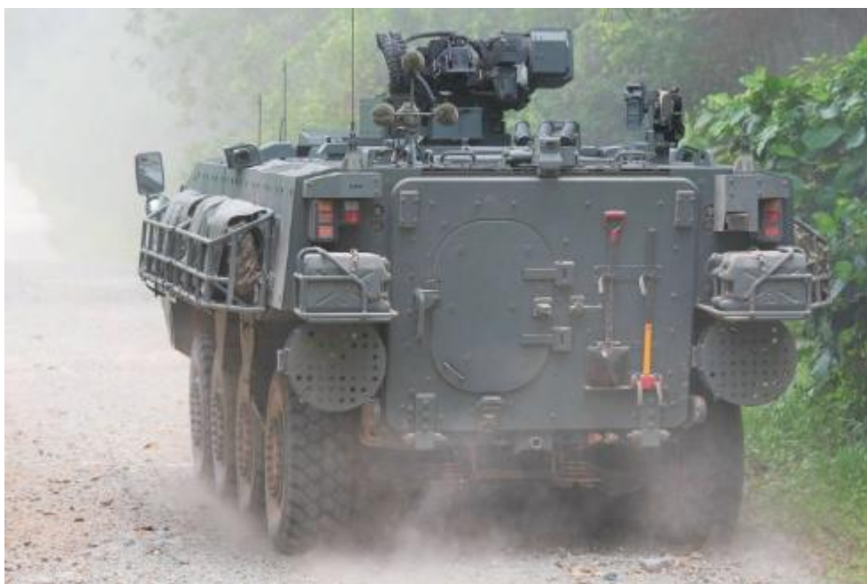
Terrex ICV carries eleven dismounts. Note the acoustic small arms detector mounted on the roof at the left rear and the manned 7.62 mm MG pintle mount on the right. The propeller shrouds can be seen either side of the rear door. (SAF) 1347975
