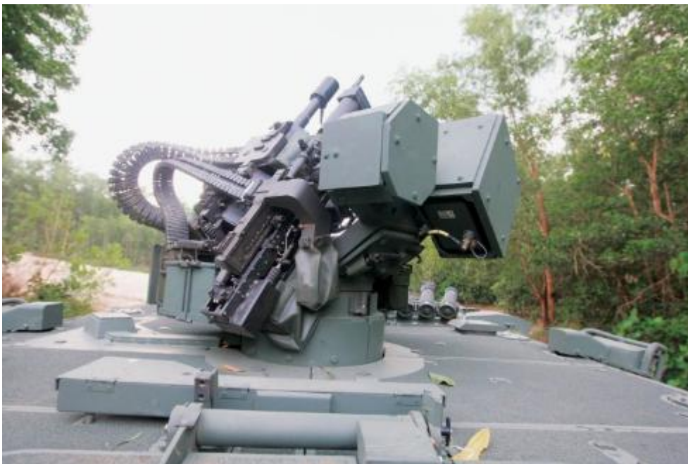
Close up of the EOS R-600 RCWS from the rear armed with 40 mm AGL and 7.62 mm co-axial MG. (SAF) 1347973
