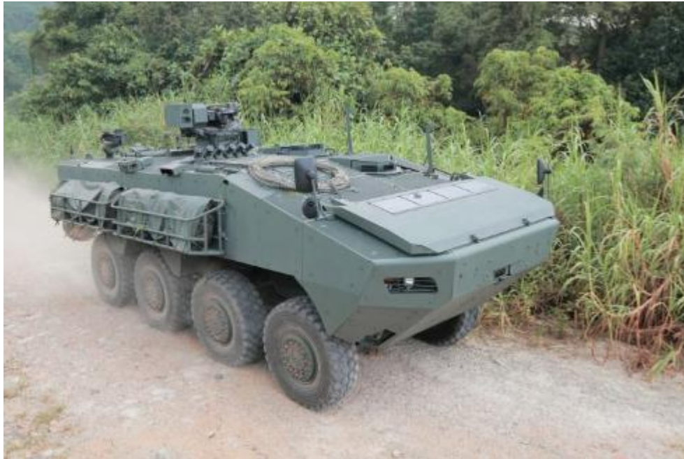
This shot clearly shows the Terrex's wire-cutters, side cameras and equipment storage. (SAF) 1347974
